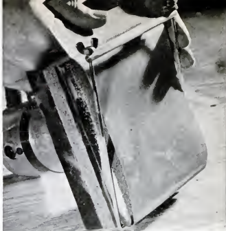
U-shaped paper clamp was bent from \frac{1}{8} " steel rod and threaded 5-40 on ends for wing nuts. Steel rod across U holds one end of paper.
